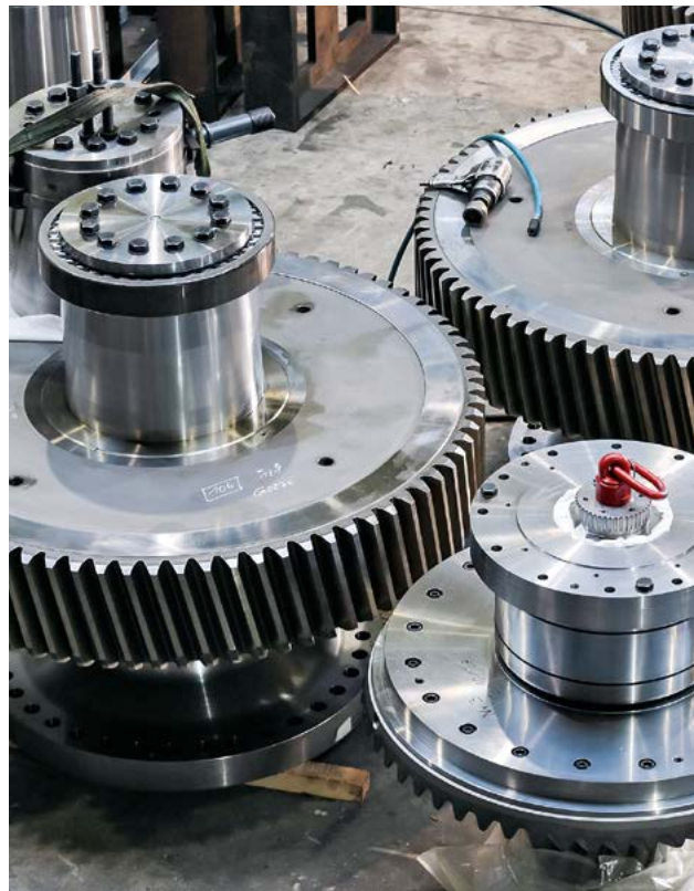
Gearwheels like these with a weight of nearly five metric tons (11,023 lb) and a diameter of 1.7 meters (5.6 ft) can easily be handled by the FAG HEATER5000
