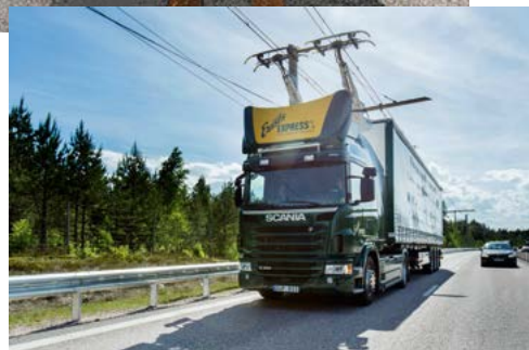
Two possibilities of range-independent electrification of trucks and buses: power rails (above) and overhead lines. Both are currently being tested in Sweden
