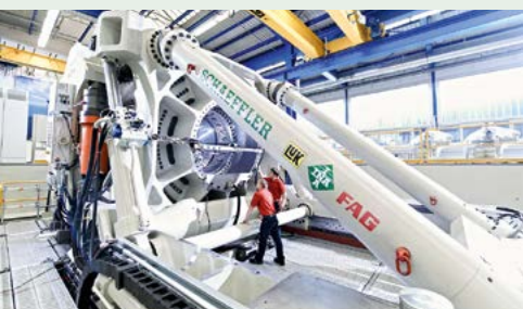
The Astraios is one of the world's most advanced, largest and most powerful test benches for large bearings
