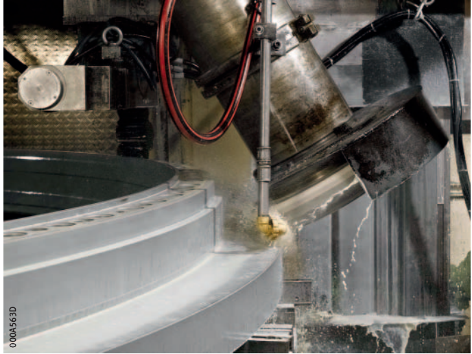
Figure 7 Regrinding of large size bearing ring
