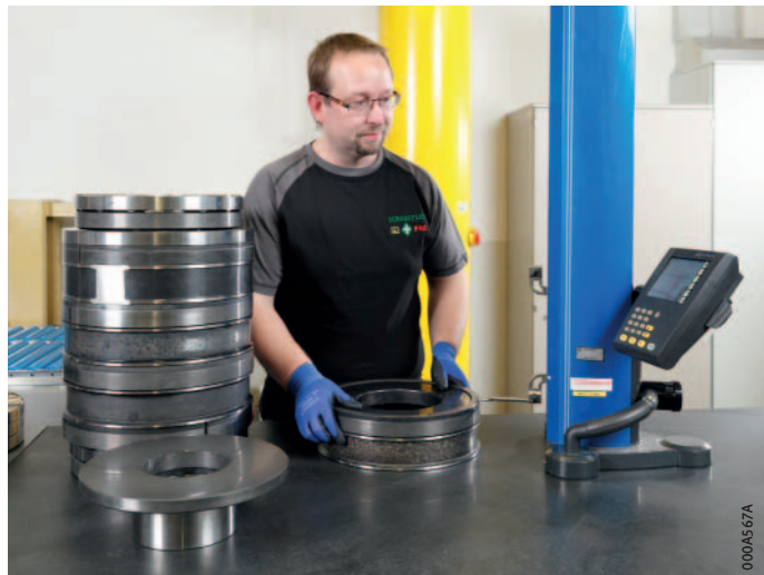
Figure 3 Measurement of a tandem bearing
