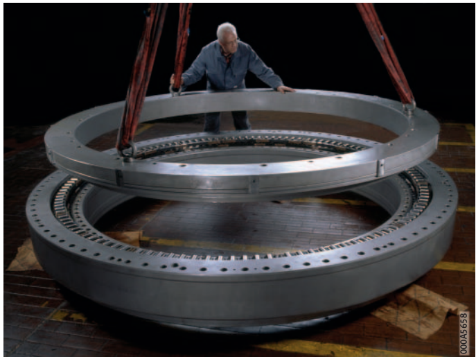
Figure 9 Mounting of a new rolling bearing ring
